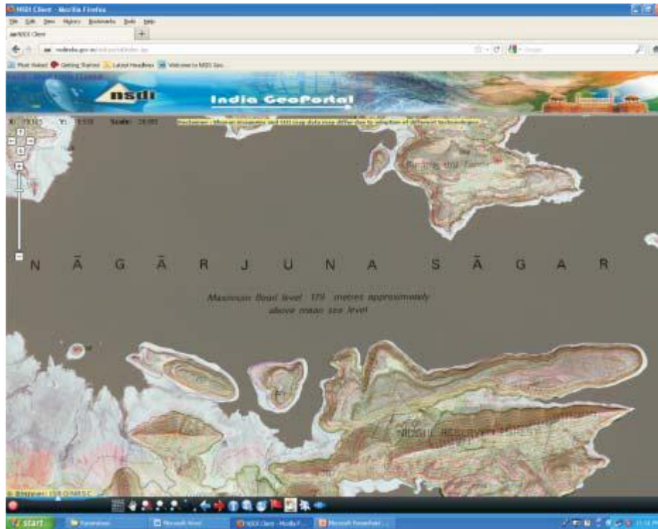
Fig. 5.50: Concurrent visualization of topographic data from SOI and IRS multi spectral imagery from NRSC on India Geo Portal
